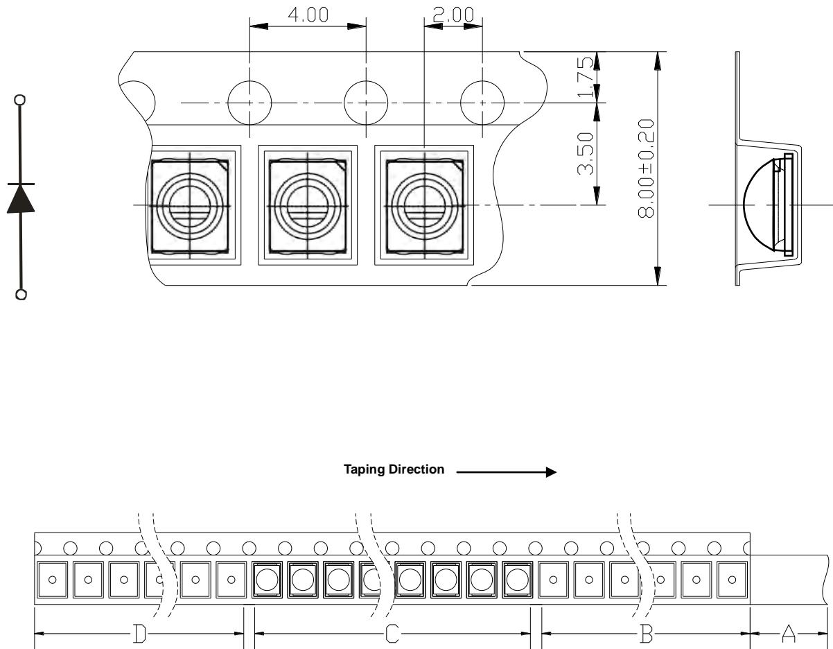
A: Top Cover Tape, 300mm; B: Leader, Empty, 200mm; C: 2000 Lamps Loaded; D: Trailer, Empty, 200mm.
